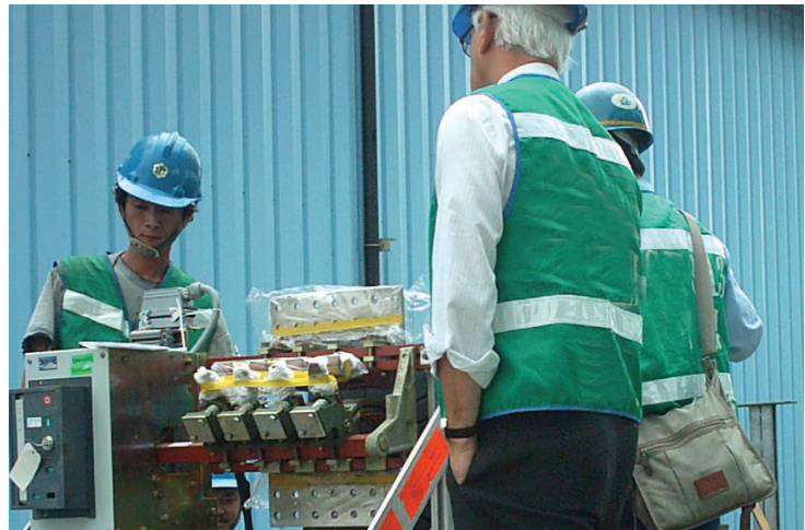
Field short-circuit test using a short-circuiting device installed on a trolley
