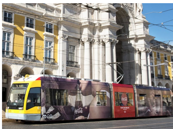
Sécheron's SPL pantograph integrated on an existing tram.
